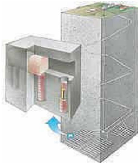
All spent nuclear fuel will be disposed of in the crystalline bedrock, 500 metres below the surface. The fuel is enclosed in copper canisters, which are surrounded by bentonite clay. The method is designed so that the waste can be left without supervision and control by future generations.
