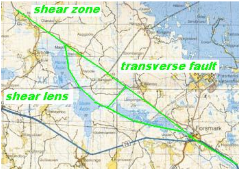
Figure 3.1. Part of the topographic map of northeastern Uppland. The topographically visible Forsmark lens has been interpreted from elevation data. The lens is down-warped in the terrain and goes diagonally across the map view. The clear transverse step in the terrain in the middle of the lens is supposedly a fault with the southeastern block down-faulted. The Forsmark lens is 10 km long and 2 km wide (from Terrängkartan ©, Lantmäteriet Gävle 2004, permission M 2004/3790).
