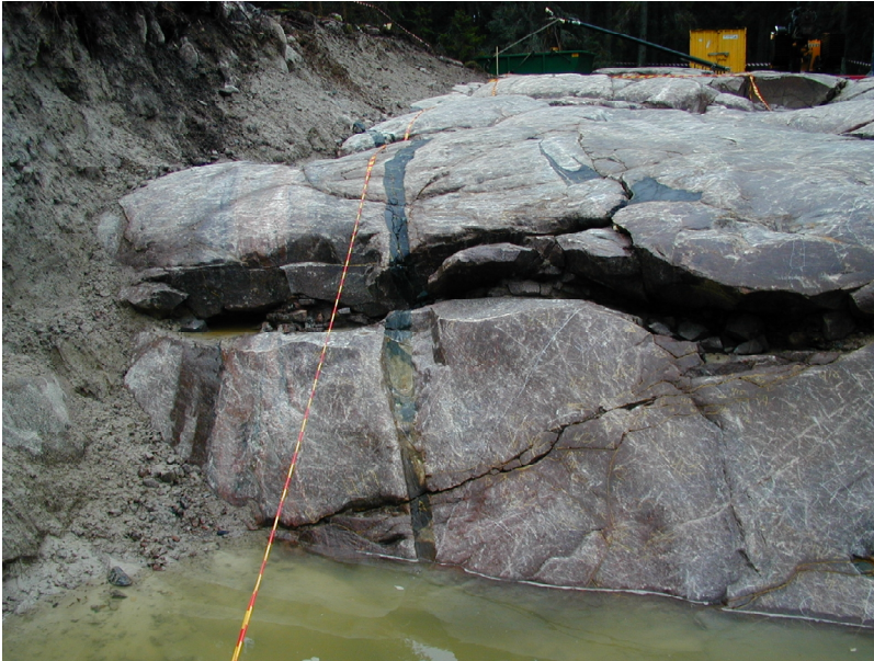
Figure 3.11. Example of a low angle fracture zone in the Forsmark area. Such fracture zones can be detected in near surface locations with ground penetrating radar and at larger depth with reflection seismic measurements (photograph by Kaj Ahlbom 2003).
